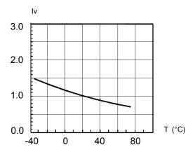
Fig. 6 Relative Luminous Intensity vs. Temperature
