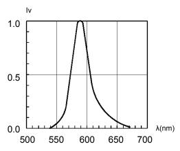
Fig. 1 Relative Luminous Intensity vs. Wavelength @ 20mA
