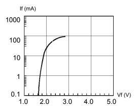
Fig. 3 Forward Current vs. Forward Voltage
