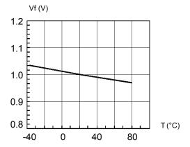
Fig. 5 Forward Voltage vs. Temperature
