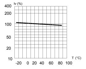
Fig. 5 Relative Intensity (%) vs. Temperature
