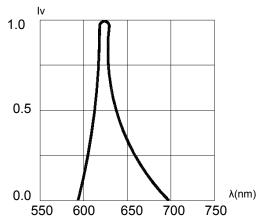
Fig. 1 Relative Luminous Intensity vs. Wavelength
