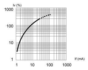
Fig. 4 Relative Luminous Intensity (%) vs. Forward Current
